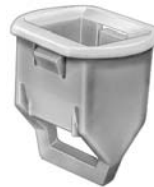
20769 (4857751AA) Natural Nylon Tail Light Retainer Head Size: 17mm x 19mm Overall Length: 21.5mm Chrysler Pacifica 2004 - On UNIT PACKAGE: 25
