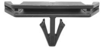
20771 (4857699-AA) Black Nylon Front Bumper Fascia To Grille Retainer Head Size: 10mm x 42mm Stem Length: 14mm Fits Into 7.5mm Hole Chrysler Pacifica 2004 - On UNIT PACKAGE: 25
