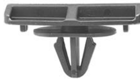
20700 (55156447-AB) Black Nylon Ground Effects Moulding Clip Head Width: 1/2" Head Length: 1-1/2" Stem Length: 1/2" Jeep Liberty 2004 - On UNIT PACKAGE: 25
